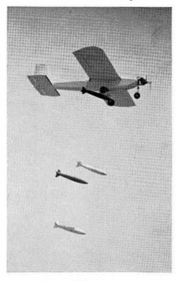
SALVO of 14-inch-long, four-ounce balsa wood test units, each painted a different bright color, are dropped on command by a radio-controlled model airplane. The units, photographed with the East Mesa tracking telescope, are targets for a study of resolution and color characteristics of all types of color film.
